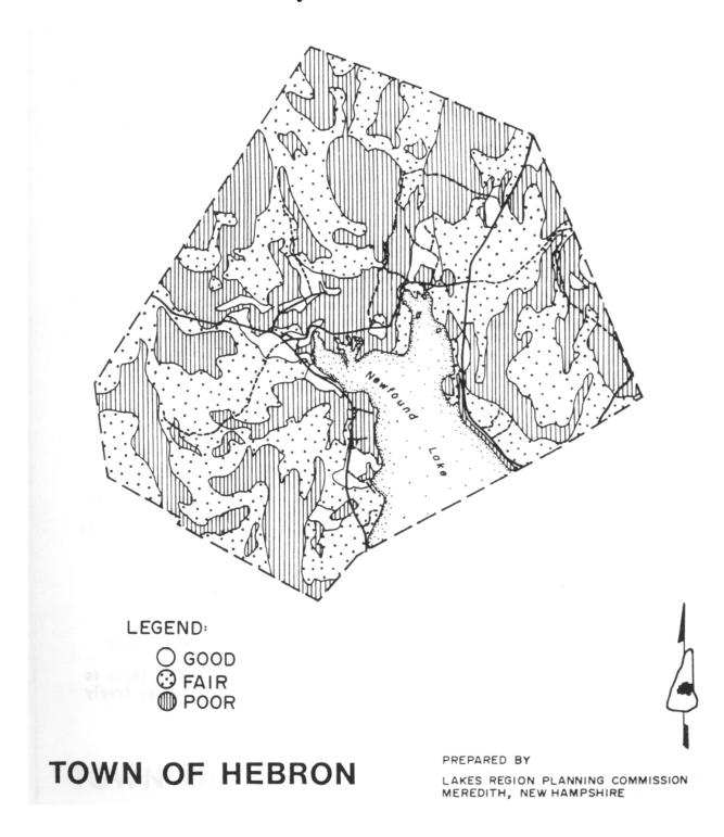
Listed below are soils found in Hebron and their limitations for road construction. The most critical soils in this group are those with potential frost action, flood hazard soils and steep slope.
