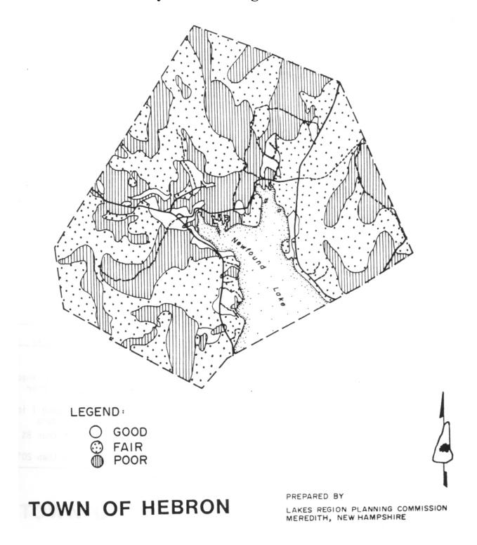
The soil must be at least five feet to bedrock to rate slight for this use. Depth to bedrock or hardpan under 40 inches is severe. A high water table will increase the severity of potential frost action.
